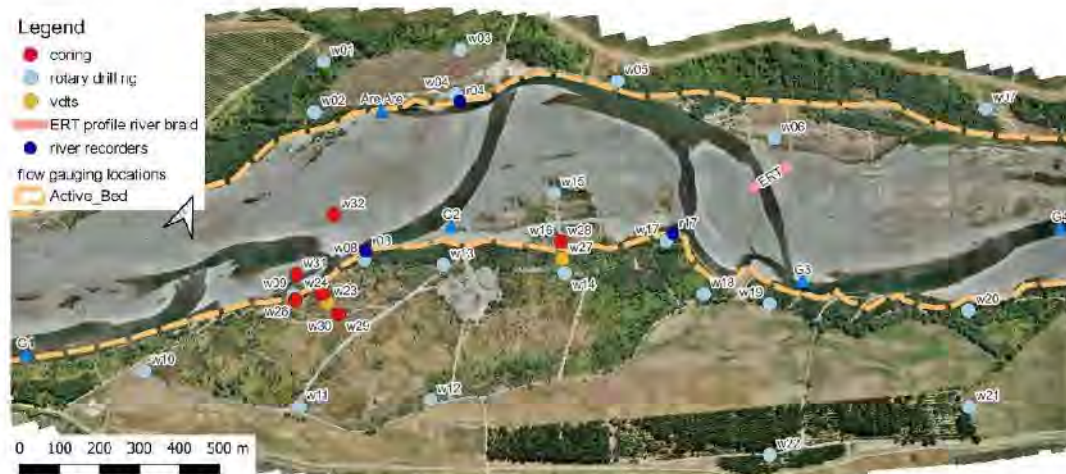
Figure 2. Wairau field site showing location of drilled piezometers (w01-w32), river stage and temperature recorders (r04, r08, r17), flow gauging sites (G1-G4), electrical resistivity tomography survey (ERT), and vertical digital temperature sensing (VDTs) cables.
