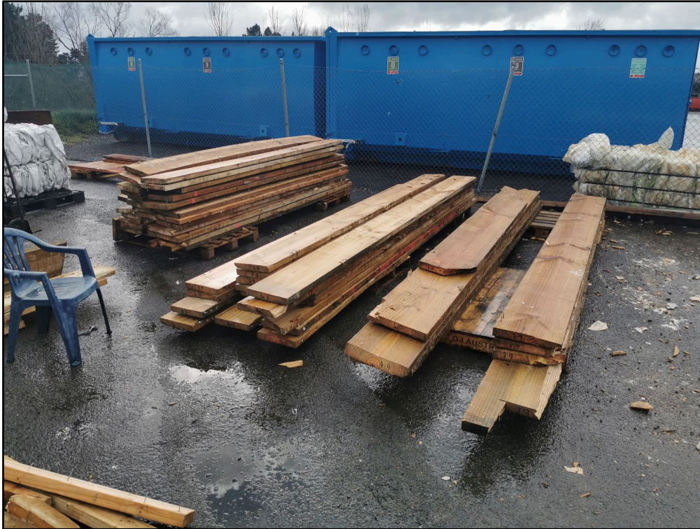
Figure 3 – Wood being reused from the Ferry terminal.
