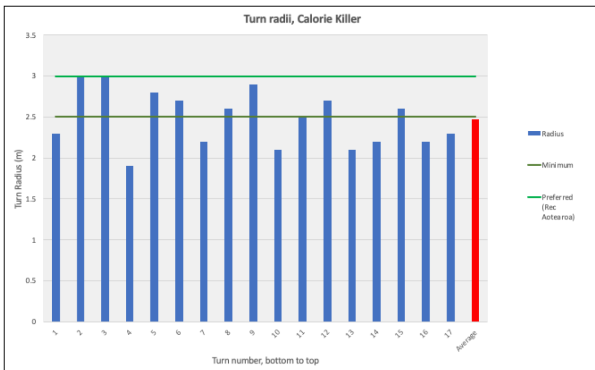
Figure 20. Turn radii on the (17) turns on Killer Calorie. On average, these are almost Grade 3 compliant. Regular maintenance is recommended and some work to ease a few, especially turn 4. (Note that we measure turn radius where we would expect competent riders of the relevant grade to be able to ride. This will not necessarily be the absolute maximum if there are rocks, roots or other difficulties.)
