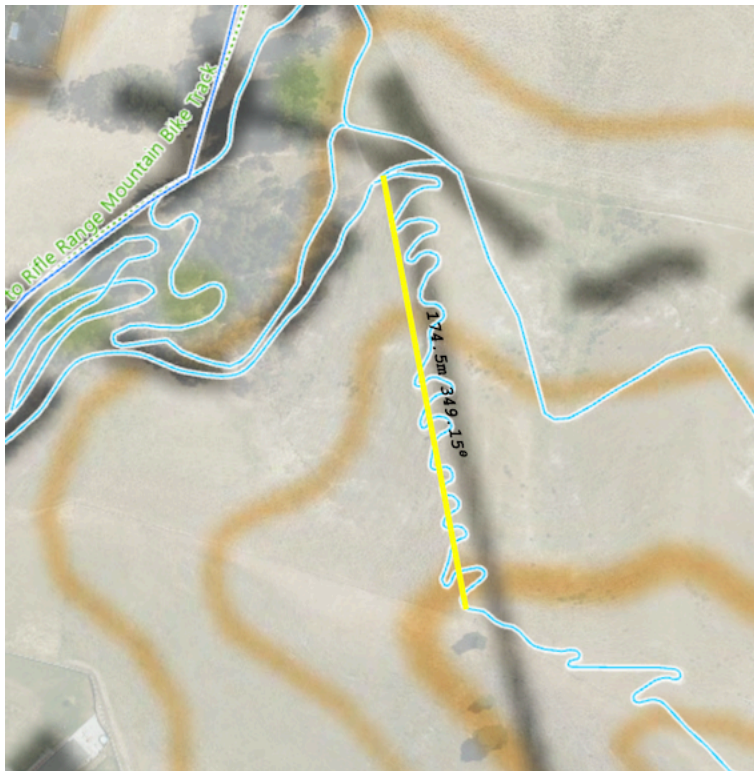
Figure 37. By way of contrast to the gentle terrain show for a proposed trail in Figure 36, this is the actual configuration of the zig-zag section of Scenic Route (Southern) above the mountain bike carpark. The slope of the yellow direct line is a whopping 18^\circ - essentially unrideable upwards and difficult terrain to build curves in.
