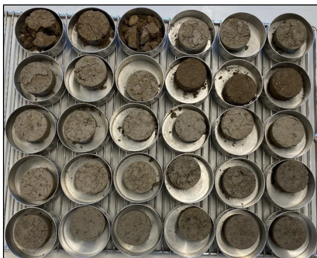
Plate 2: An example of dried cores inside their extraction rings following oven drying. Credit: A. Van de Laar, Manaaki Whenua Landcare Research.
