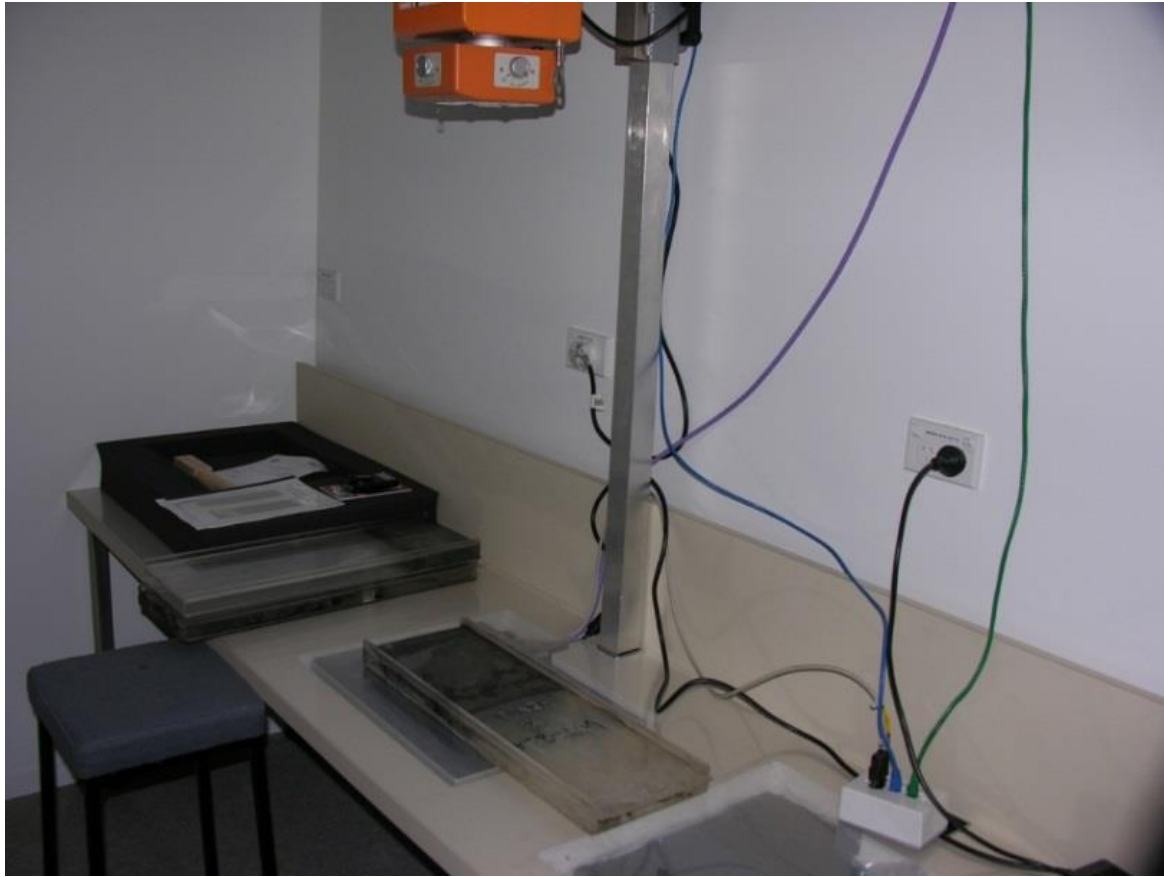
Figure E-1: NIWA digital x-ray system. A sediment slab mounted on the x-ray detector plate ready for imaging. Photo: Ron Ovenden, NIWA.
