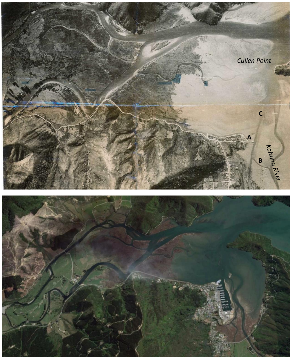
Figure 1-15: Aerial photographs of Havelock Estuary, 13 April 1942 and 31 December 2015. (top) 1942: image shows the wharf at the end of Cook Street (A), constructed channel connecting the Kaituna River with the wharf area (B); and the channel that now forms the present-day entrance to Havelock Harbour; (bottom) 2015: present-day wharf and marina facility, with the dredge-spoil island immediately north of the marina entrance. An area of post-harvest pine forest is visible on the hillslopes flanking the northern side of the Pelorus River mouth. Image elevation: 6.7 km. Source Google Earth.
