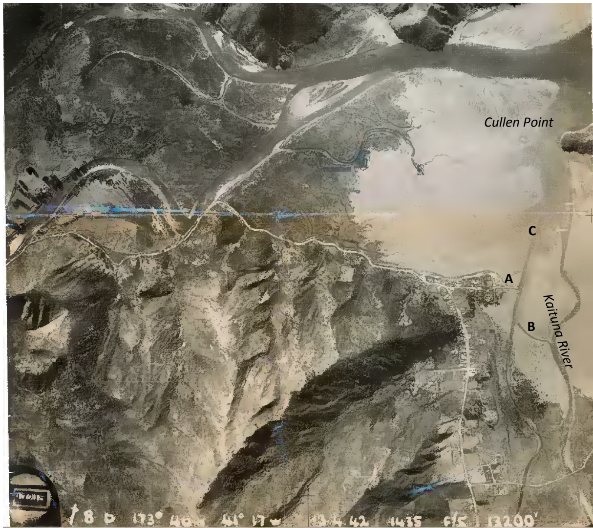
Figure 1-2: Havelock Estuary, 13 April, 1942 showing: A, the wharf at the end of Cook Street; B, the man-made channel connecting the Kaituna River channel with the wharf; and C, the channel that now forms the entrance to Havelock Harbour.
