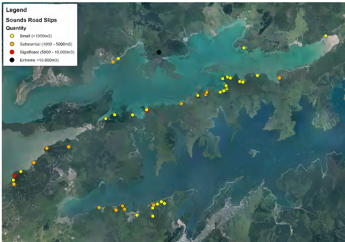
Figure 1-6: Slips that entered coastal waters associated with the transport road network on Queen Charlotte Drive (bottom centre – 12 dots) and the Kenepuru Road. Source: Miller (2015).
