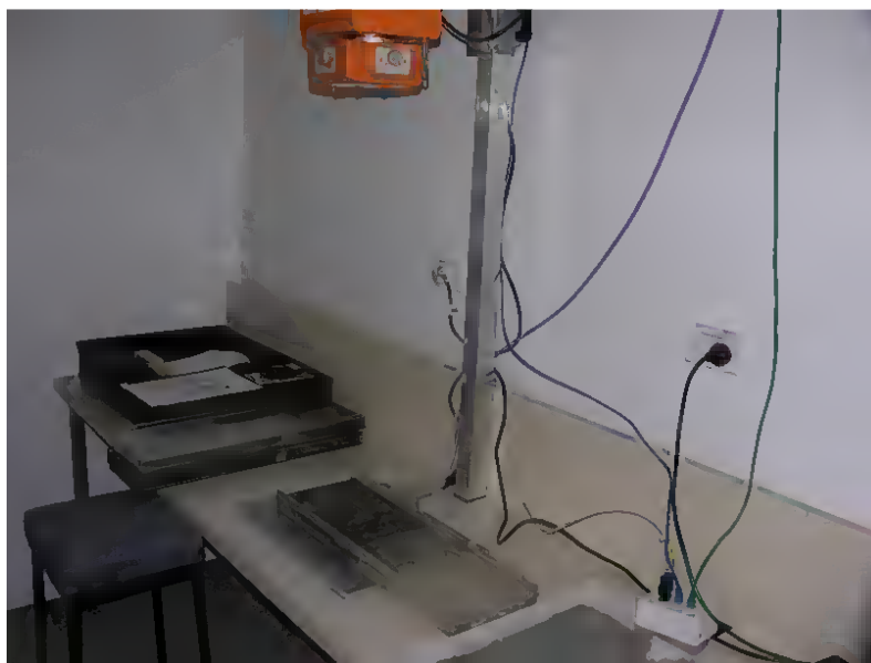
Figure 2-6: NIWA digital x-ray system, with a sediment slab mounted on the detector plate ready for imaging. (Photo: Ron Ovenden, NIWA Hamilton).
