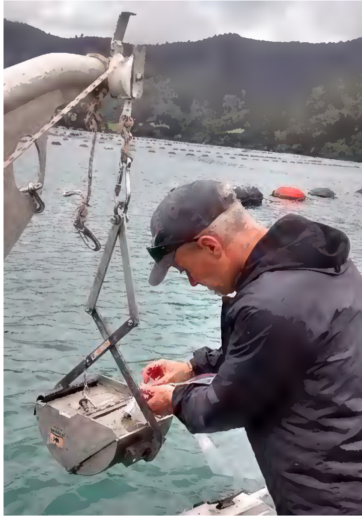
Figure 2-3: Example of marine sediment grab sampling beneath a mussel farm, inner Kenepuru.
